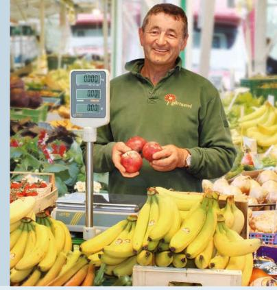
Price computing scales are used anywhere where the price of goods is calculated dependent on the weight of the goods. These scales must be verified in accordance with European Directive 2009/23/EEC. Usually, these scales are in verification class III.
