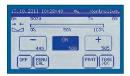
Weighing with tolerance range (checkweighing): a visual and audible signal helps with portion division, dispensing or grading
